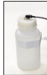
Fig. 5: Check of condensate collection vessel
