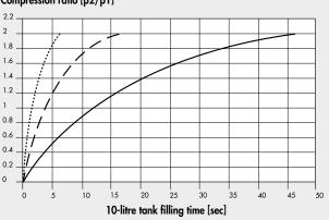
The graphs refer to the filling of a 10-litre tank and show the ratio of outlet to inlet pressure (= p2:p1) as a function of time (sec).
